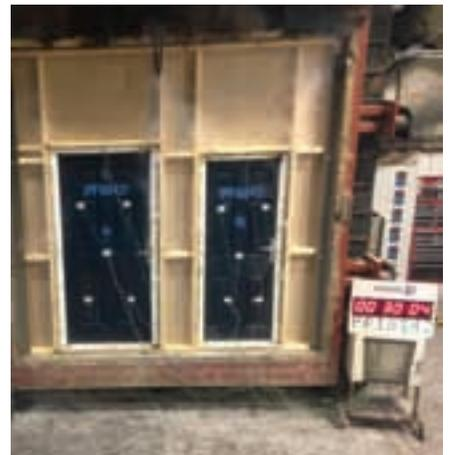
retardant glass and door panels and feature a graphite intumescent strip which expands with heat within the specially reinforced frame to create a 30-minute fire rating (complying with the requirements of BS476 FD30 Pts 20 and 22).
